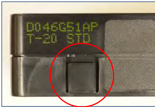
Figure 5 – Write-Protect Tab
