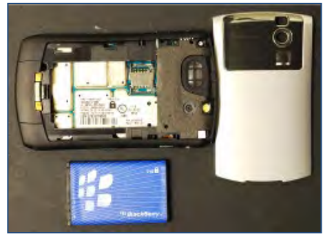
Figure 1 – Battery Removal
