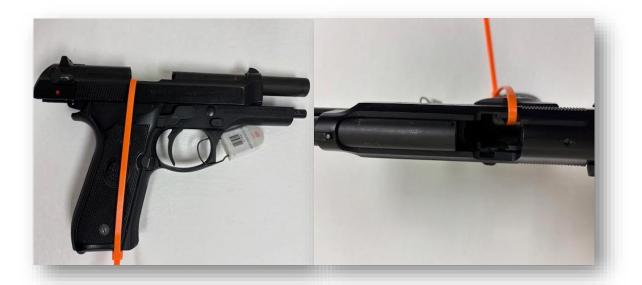
Alternatively, after removal of the magazine and clearing of the chamber, a plastic zip-tie can be run through the empty magazine well and out the ejection port.
