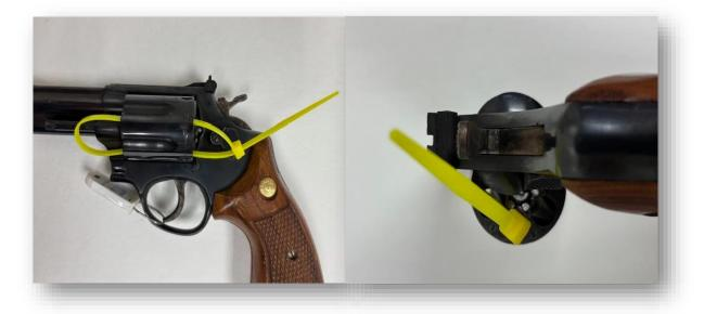
For revolvers, after all chambered cartridges have been removed, a plastic zip-tie can be looped through two empty chambers, preventing the cylinder from closing.
